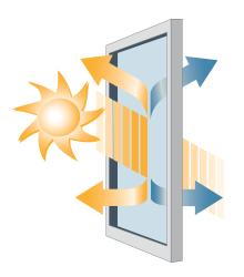
In warm weather, Low-E 180 glass reflects the sun's energy and prevents it from entering the home. In cold weather, Low-E 180 glass reduces the amount of heat lost by reflecting it back inside.
